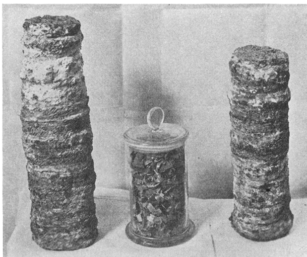
FIG. 3. Two calcium cylinders or rods produced in cell shown in Fig. 1. Also a glass jar of calcium metal shavings.
