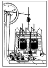
*Figure 2*. Electrocapillary motor; Ref. 5, p 522.
