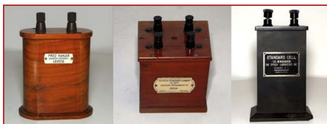
FIG. 6. Assorted standard cells. In the middle are two cells in one container for comparison (photo author).
