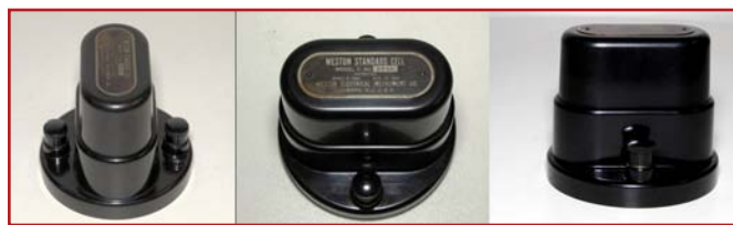
FIG. 4. Cell manufactured by Weston Electrical Instrument Company—the unsaturated version (circa 1950s) (photo author).
