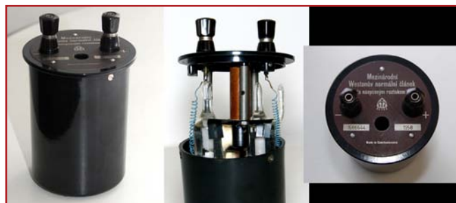
FIG. 5. The standard “International Weston normal cell with saturated solution” manufactured by Metra, Czechoslovakia (1958) (photo author).
