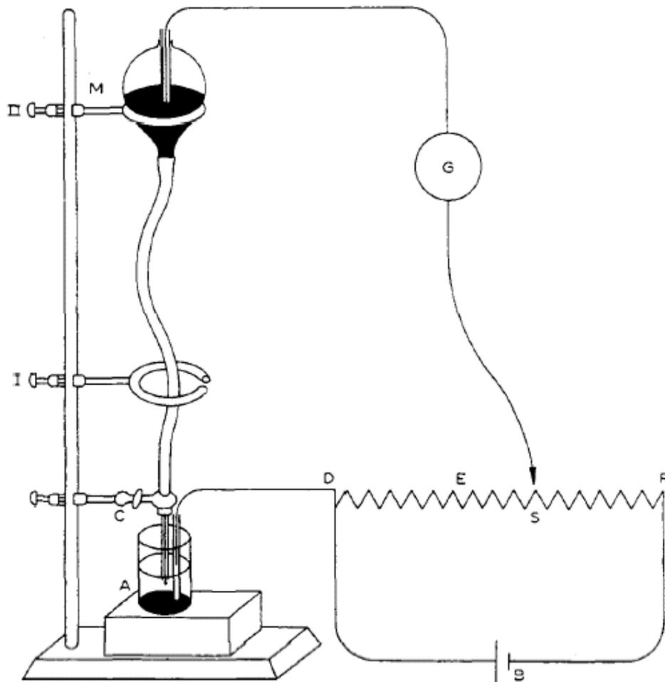
Fig. 2. Simplest polarographic arrangement.
