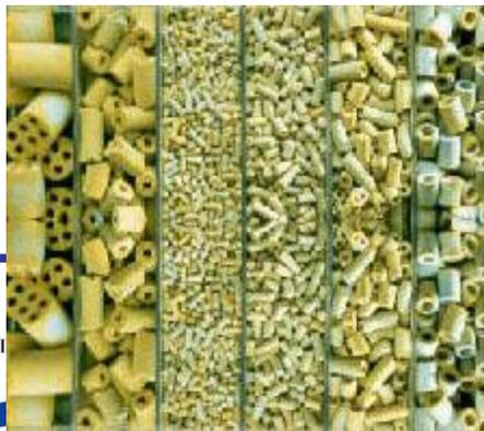
Thermostable catalyst ICT-12-40 for of toxic organic impurities and carbon monoxide in industrial waste gases.
