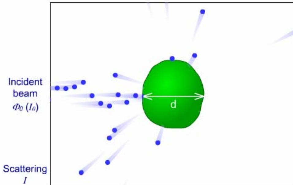
$$\sigma [\text{cm}^2] = \frac{I [\text{c}^{-1}]}{\Phi_0 [\text{cm}^{-2}\text{c}^{-1}]} \quad \text{cross-section}$$
