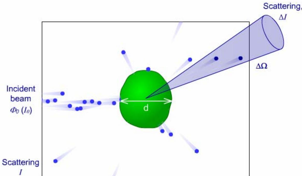
$$\frac{\Delta\sigma}{\Delta\Omega} [\text{cm}^2] = \frac{\Delta I [\text{c}^{-1}]}{\Phi_0 [\text{cm}^{-2}\text{c}^{-1}]} \quad \text{differential cross-section}$$
